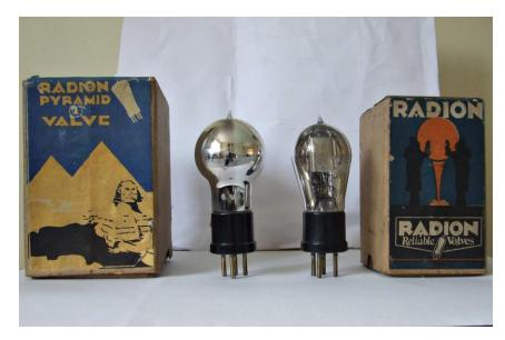
It is believed Radions made most of their own machinery to process the intricate assemblies. required This the replacing of the hairthickness tungsten filament wire bur it was not an easy task. The bulb, already under high vacuum, had to opened in a high temperature flame at opposite ends across the bulb (in one way), the filament replaced and
