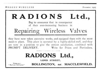
Radions were set up initially to repair valves. Bright emitters were repaired for 6/6d (32½p) at a time when new ones cost about 8/- (40p) and dull emitters such as the BTH **B5** were converted to emitters. Radions, like others in the repair business, did not repair using thoriated tungsten 'dull emitters', possibly because only lamp grade tungsten wire was available at a price but more likely because it would take time to master the use of thoriated tungsten wire.
